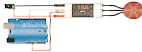
Fig 3. Arduino Interfaced with ESC
